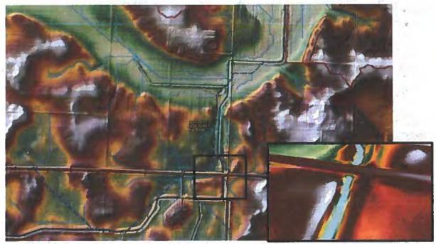
Figure 2. Example of "digital dams" existing in LiDAR datasets that impede flow paths through water conveyance infrastructure.
